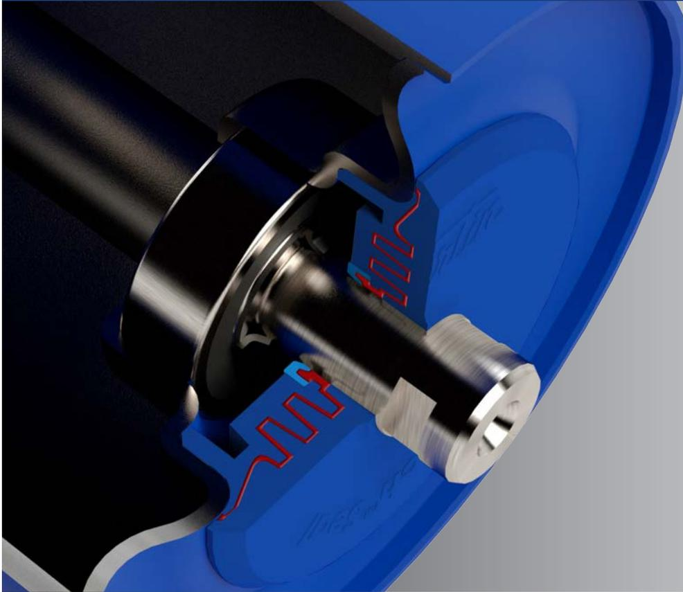
**Martin Triple Labyrinth Seal design offers the following bearing protection**
